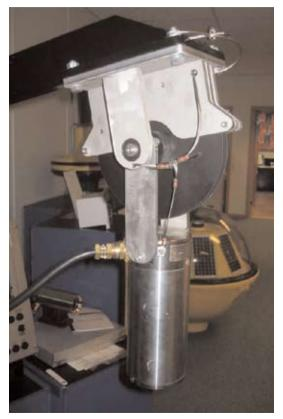
There have been several cases where a crane camera has been hit by the crane during lifting operations. Since bolts through the attachment bracket would be unable to withstand the forces generated by a collision of this kind, it is vital to equip crane cameras with two anti-fall barriers.
